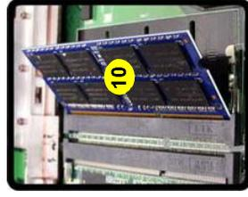
5. Pull the latches to release the second and third modules if necessary.
